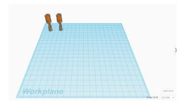
Now, drag over a box hole piece. Resize it so that it is 5mm tall and large enough in length and width to completely enclose your object:
