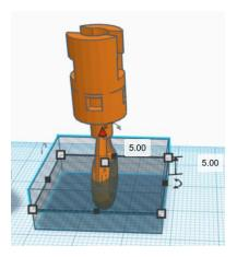
Duplicate it six more times until your entire object is completely enclosed by a stack of 5mm tall hole pieces:
