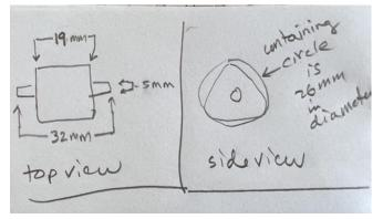
The part has a diameter of 26 mm when viewed along its axis (right hand diagram above). The pins that stick out on the sides are 5 mm in diameter and stick out 32 mm side to side (left hand diagram above). Watch this short video to get a 3D view of the part.
