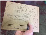
This is done by breaking the nodes so there are little parts that aren't cut through by the laser. You can see the little breaks in the paths above in the Inkscape screen shot. Each piece above has one or more breaks so that it won't fall out until someone purposefully pops the piece out to build the project.
