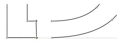
Repeat on the other side and you have made the D laser-cuttable:
