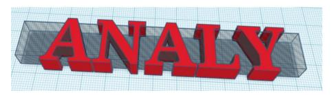
When I group those parts and check the new volume of the object, it was lowered to 1800 cubic mm. That's a huge reduction (from nearly 7500 down to 1800 in one move!). See the resulting object on the next page.
