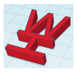
Next create a cylinder that is 5 by 5 by 20 and place it in the center of your letters (it has to be overlapping with part of a letter, it can't be in a hole spot, you may need to add other connectors or move it from the center to make this work.) Here is what I did:
