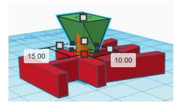
That is a triangle piece, flipped over, that is 15 by 10 and 10 mm tall. Line it up so that the big flat part is even with the cylinder (see how you can see the circle on the top of mine above?)
