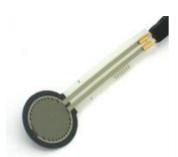
This thing is a resistor. When you press it, its resistance changes, which can be sensed by an Arduino. It's a lot like the LDR (light dependent resistor) except that it's the force you apply to it that changes its value instead of light.
