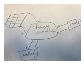
Create your diagram electronically (Tinkercad or Gravit). The image above is just showing you the information you need to include and how it might be arranged (there are four parts, plus wires.)
