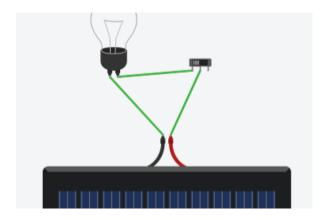
To connect wires between the objects to make a circuit you click on a terminal (one of the little tabs that sticks out from an object) and drag over to the tab of one of the other objects and click on the place you want the wire to go. If you make a mistake, just delete the wire and try again.
