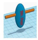
The blue part is not touching the work plane. The horizontal bar is all overhang. 3D printers are OK with a little overhang (think the letter Y, not the letter T), but not a straight bar hanging out of something. Also, long thin things sticking out or up often do not print well. Finally, the text simply will not print well, it almost never does, unless you are printing very large things and on a face-up surface.
