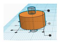
Next, make a box that is 15 by 15 by 7.5. Bring it over so that it is lined up with the two cylinders like this:
