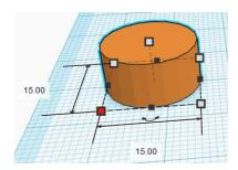
Next, make a cylinder that is a hole piece and make it 15 tall and 4 by 4 around.
