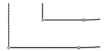
Either select a node, or add your own by double-clicking on the line then break the path using the correct icon from the toolbar:
