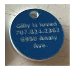
The text must be black, with fill turned on, black stroke, and thick enough to actually raster. Same for images. Here are some good and bad examples:
